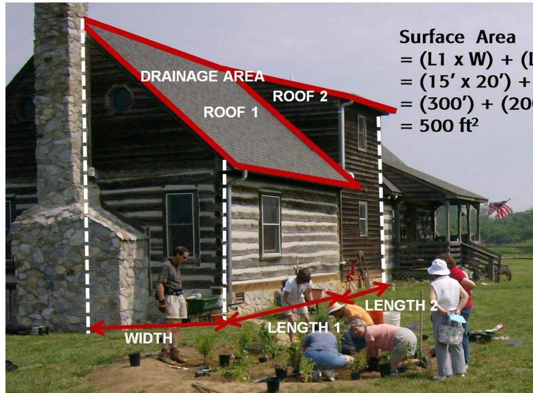
$$\begin{aligned}\text{Surface Area} &= (L1 \times W) + (L2 \times W) \\ &= (15' \times 20') + (10' \times 20') \\ &= (300') + (200') \\ &= 500 \text{ ft}^2\end{aligned}$$
